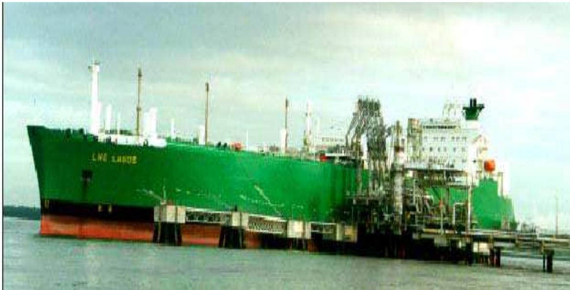
**Figure 16. LNG Lagos - Membrane Type LNG Carrier**
