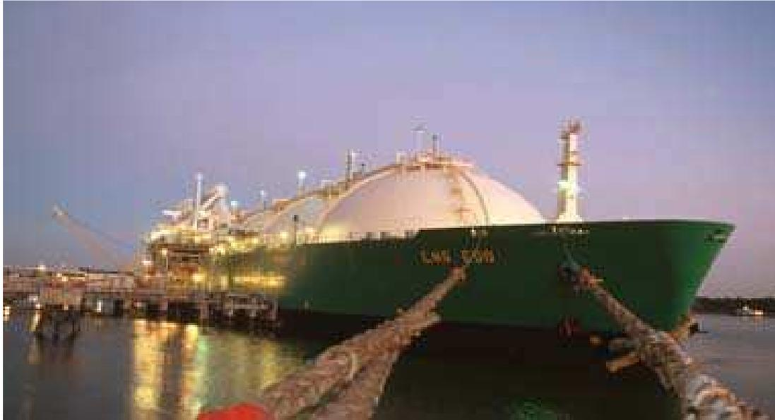
**Figure 15. A Spherical Tank**
